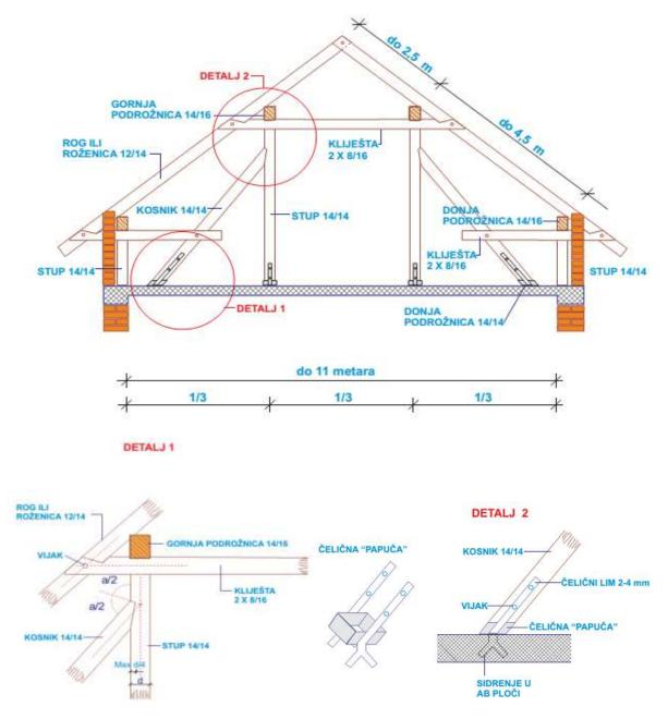
Queen truss can have a range between 7-12m. The minimal gradient is  $25^{\circ}$ - $30^{\circ}$  and maximal length of rafter is 7-7.5m.
