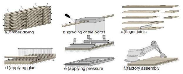
Figure 4, manufaturing of cross laminated timber
