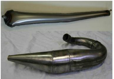
Figure 4. Parts formed by hydroforming of welded sheets
