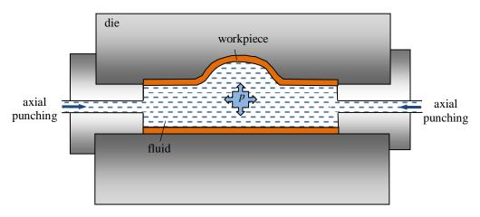
Figure 5. Hydroforming of tube
