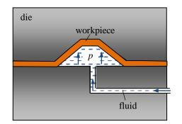
Figure 1. Sheet metal deep drawing by hydroforming
