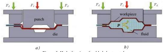
*Figure 3. Hydroforming of welded sheet metal* Hydroforming process of welded sheet metal comprises following phases: a) Positioning of welded sheets in mould and filling space between sheets by fluid under pressure, (performing phase).
