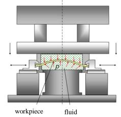
Figure 2. Sheet metal stretching by hydroformig
