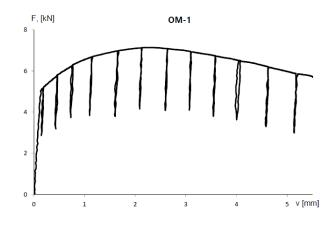
Figure4: Unloading compliance toughness test record
