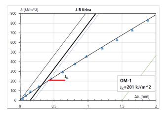
Figure 5: Calculated J-R curve with critical value of  $J_{Ic}$
