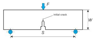
Figure3: Single-edge notched bend (SENB) specimen
