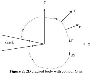
Figure 2: 2D cracked body with contour G in counterclockwise direction
